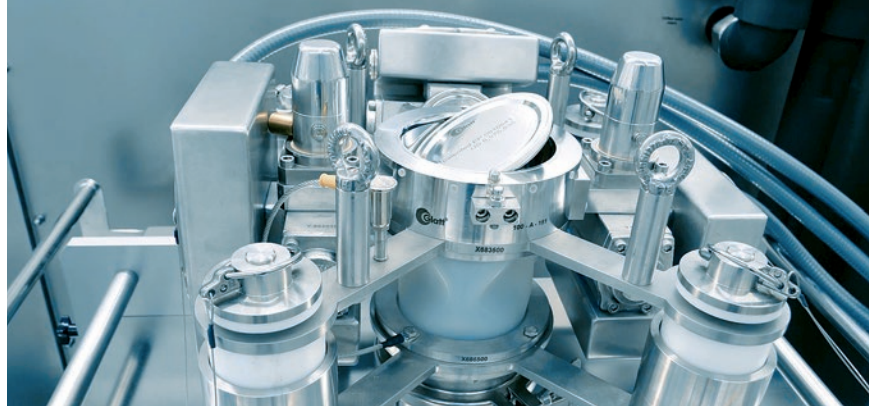
A Glatt containment flap (active/passive) type TKS is used for product feeding. Here the active flap in the hopper opening.
